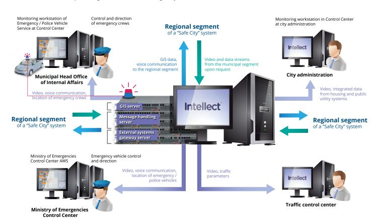
The managing company monitors the technical aspects of the system, ensures camera uptime, and calculates the amount due for technical services after the end of each billing period. Camera status is monitored by means of automated quality loss/sabotage detection tools.
