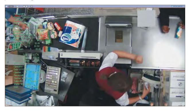
Both in real time and during later video viewing, the operator sees video of a buyer transaction with text (captions) containing information at the bottom of the screen. This information includes the text of the receipt and events at the cash register that are not displayed in the receipt, such as opening of the cash drawer or manual entry of a product code. This approach allows seeing the full picture of events occurring at the point of sale.
